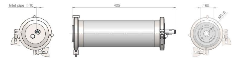
An example of pneumatic motor with case configuration : weight 10 kg, consumption 8,1 l/s
